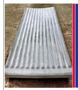
Part of the Trona refining process involves rotor blades accelerating the sorbent particles against the teeth of components called cutter blocks to break the particles apart. SCP provided custom cutter blocks made out of our SCProbond™ 'N', nitride bonded silicon carbide after previous materials could not meet run-time requirements.
