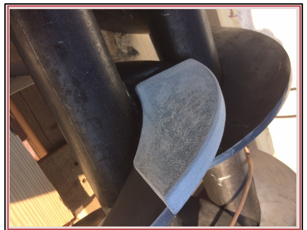
Custom Screw Conveyor Flight Plate Installed with SCProbond™ epoxy
